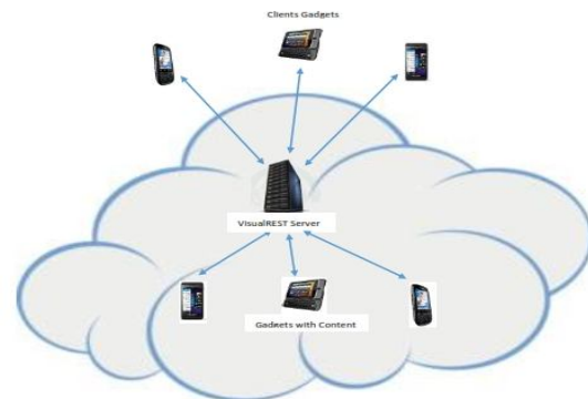
Fig. 2: Architecture for managing content in a cloud of mobile gadgets
